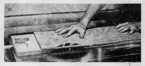
'liding table idea plus anchor points to hold the work makes a good set-up for ripping raw edges.
