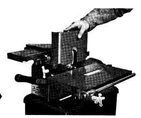
Invert the guard which was previously removed from under the saw table and place it over the top of the saw blade and retighten the small wing nuts.
