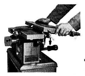
Grasp Saw Table at the front and rear and tilt up the edge nearest the planer to about twenty degrees so that the edge will clear the saw teeth.
