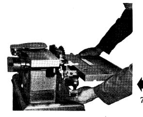
Providing the nuts have been loosened sufficiently the saw table can now be lowered to the bottom of the travel of the secondary slide and the two hexagon nuts relocked, using the same spanner but working from the underside of the saw table as shown.
