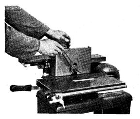
Hold the control handle, release the wing nut lock, lower the table to the bottom of its travel. Insert a standard  $\frac{1}{2}$  shank boring or mortising bit, as the case may be, into the end of the saw spindle. Using the "tommy bar" supplied, fit it into the cross drilled hole in the saw spindle so as to prevent the spindle from rotating when the collet nut is lightly tensioned with the spanner provided.
