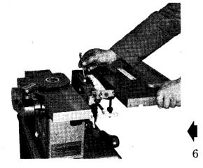
With the spanner provided loosen the two hexagon nuts visible down behind the saw blade, while at the same time supporting the weight of the table with your other hand.
