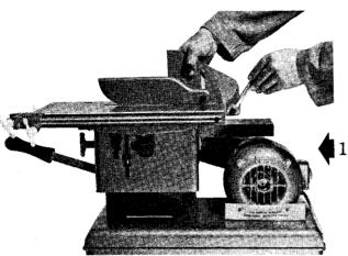
Release wing nut lock and raise tables to their full height by means of the main control handle, retension wing nut lock so as to keep the tables in the full up position. (The wing nut lock referred to is the one illustrated as being under the tables just above the control handle where this handle enters the machine.) Loosen the bolt holding the rifing knife to the rear of the saw table and lift the rifing knife, and the saw guard as one complete unit, clear of the table.
